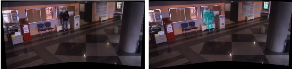
Figure 24. Example of an incoming frame included on the panoramic and the result of the background subtraction algorithm.
